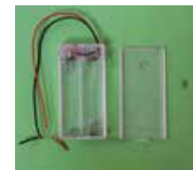
2. Use screw driver and take the lid off from the battery holder.
