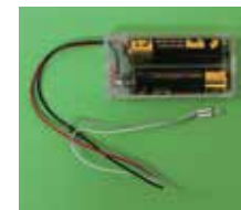
4. Connect the red wire to grey wire. Connect the black wire to white wire.
