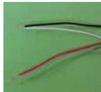
Do the same on the white wire. Remarks: Tie a knot at the end of the grey wire to differentiate the polarity.
